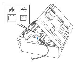
Carefully route the network cable through the trench and out the back of the machine. Then, connect the cable to your network.
